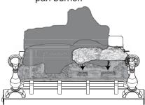
4.2.4 Position the slotted cavities on the bottom of log #3 onto the slotted projections shown. The charred face should be facing in.
